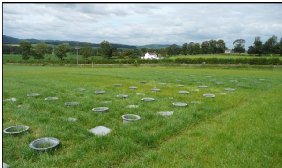
Figure 2. Chambers used to measure nitrous oxide emissions at Crichton.
