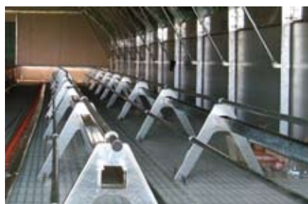
Fig. 3: A-frame style perch, incorporating feed track (courtesy of Newquip/Big Dutchman)
